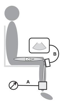
**Figure 1.** Test setup for the biomechanical measurements of patellar tendon properties. The subject was positioned in a rigid chair with hips and knees flexed at a 90° angle. *A*) The lower leg was fixed with a strain gauge around the ankle. *B*) An ultrasound probe was positioned over the patellar tendon, visualizing the patella, the entire tendon, and the proximal tibia. Recordings were made while the subject performed a ramped 10 s maximum isometric knee extension.
